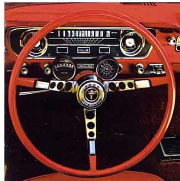
Rally Pac (tachometer and electric clock)
